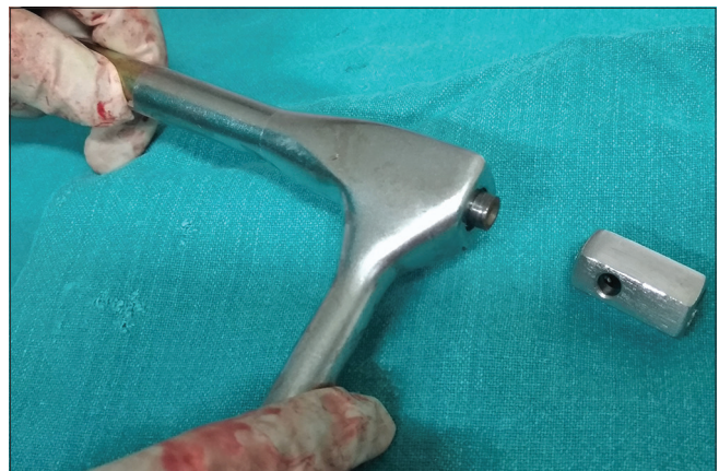
Figure 5: The part of proximal jig for femoral nail broken soon after mounting the nail. The another jig arrangement delayed the surgery
