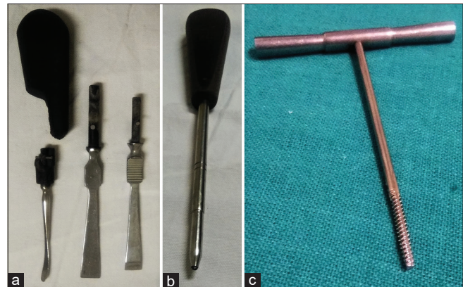
Figure 2: The periosteal elevators with wooden handle broken and its metallic part separated (a), the screw-driver with broken tip (b). The bone tap broken through its thread part (c)
