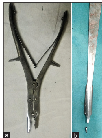
Figure 3: The broken tip of the bone nibbler (a) and the bone lever (b)
