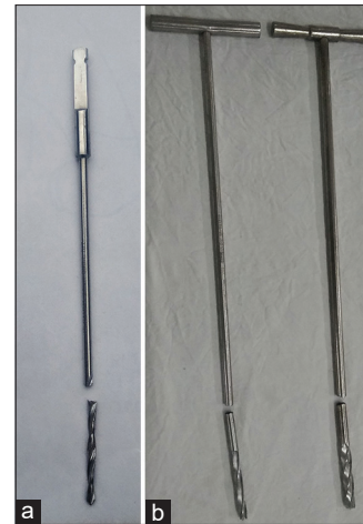
Figure 1: The broken drill bit through proximal threads (a) and two manual intra-medullary reamers broken above the cutting thread region (b)
