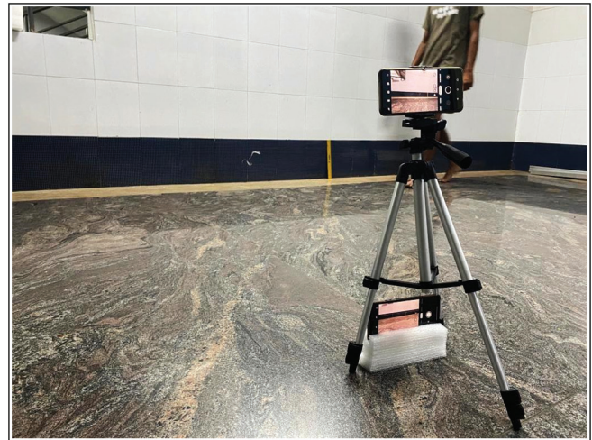
Figure 2: Video recording setup used in this study. The pathway length was 5 m with the recording camera placed at a distance of 3 m from the subject (reproduction size at column width)
